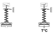
Set point and reset point must be between 10% and 90% of the selected scale.
