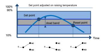
A vapour filled flexible sensing element actuates a microswitch by means of a piston. The set point is adjusted by means of a compressible spring installed in opposition.
