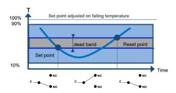
Set point adjusted on raising temperature 100% 90% Set point Reset point 10% Time A vapour filled flexible sensing element actuates a microswitch by means of a piston. The set point is adjusted by means of a compressible spring installed in opposition.
