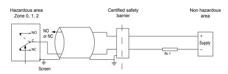
For max. ambient temperature according to temperature classes T5 and T6 refer to technical data on page 1. The installation must be made in an intrinsically safe circuit whose certified electrical safety parameters do not exceed any of the values  $U_{max}$ ,  $I_{max}$  and  $P_{max}$  given in the electrical data on page 1.
