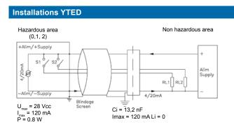
In area 0, the combination of the pressure switch and the safety barrier must be covered by a calculation checked by an approved body. For the application in Ex zone you have to respect the conditions mentioned in the ATEX Type Examination Certificate (LCIE 03 ATEX 6300 X).
