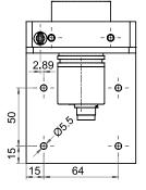
All details in mm and dependent on the encoder configuration.
